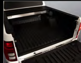
Under Rail Tub Liner
